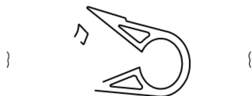
Figure 1 — Design of a pinch clamp (schematic)
