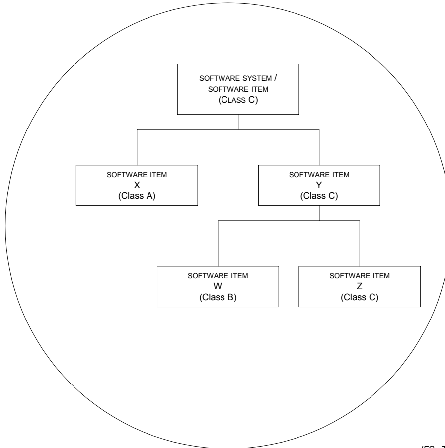
Figure B.1 – Example of partitioning of SOFTWARE ITEMS
