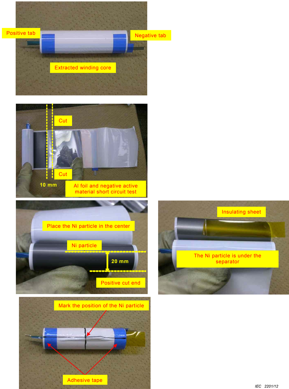
Figure A.5 – Disassembly of cylindrical cell
