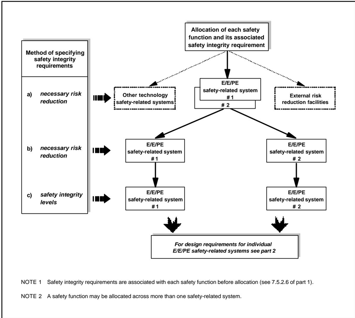
**Figure A.3 — Allocation of safety requirements to the E/E/PE safety-related systems, other technology safety-related systems and external risk reduction facilities**
