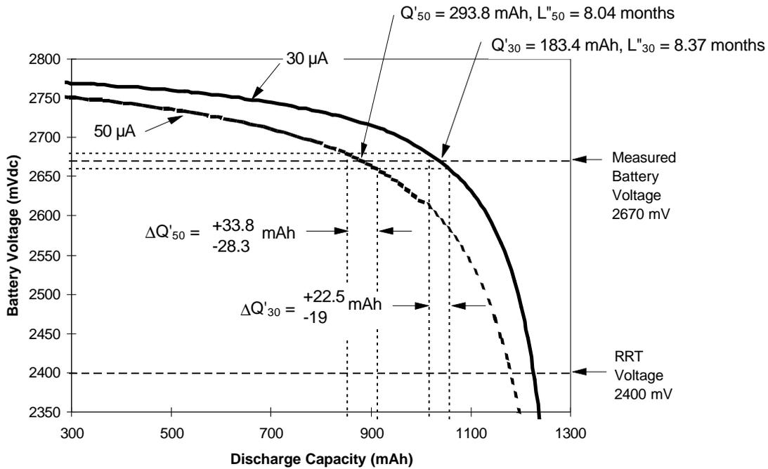
**Figure C.3—Load voltage-capacity for a specific lithium/iodine battery discharged at 30  $\mu\text{A}$  and 50  $\mu\text{A}$**
