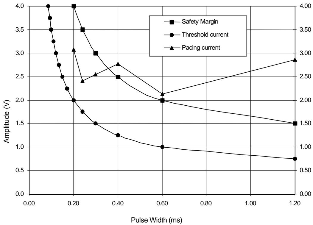
**Figure A.8—Threshold, safety margin, and pacing current**
