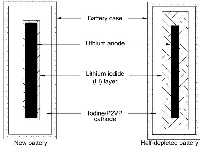
**Figure A.3—Cross-section of new and partially depleted lithium/iodine pulse generator batteries<sup>4</sup>**
