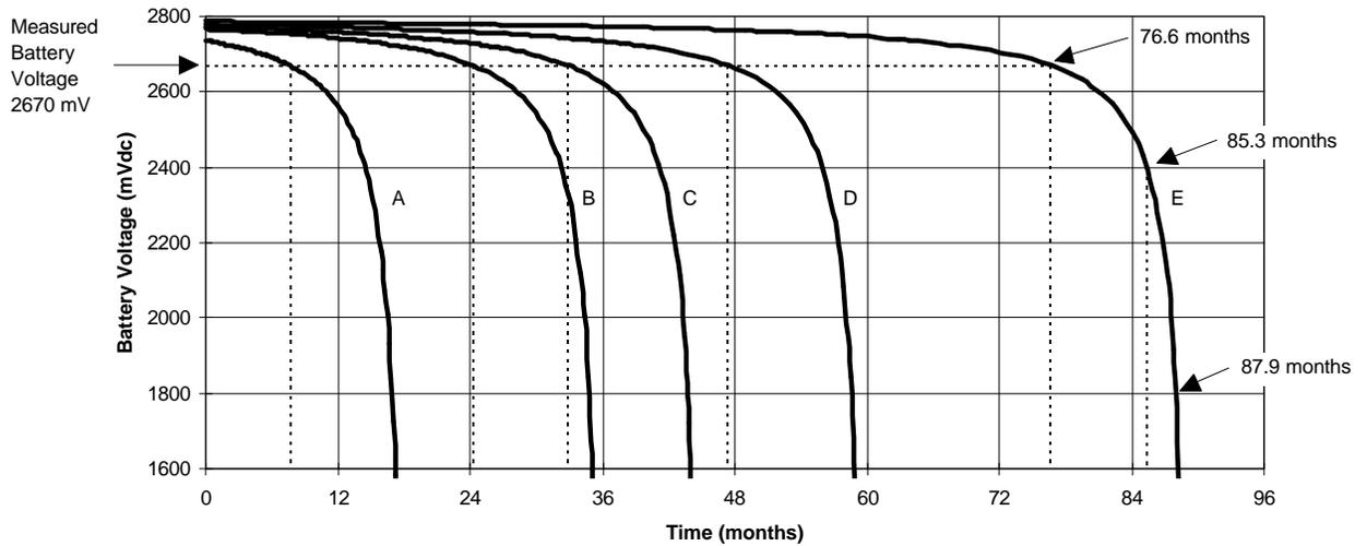
NOTE—Curve A = 100  $\mu\text{A}$  , curve B = 50  $\mu\text{A}$ , curve C = 40 $\mu\text{A}$ , curve D = 30  $\mu\text{A}$ , and curve E = 20  $\mu\text{A}$ .
