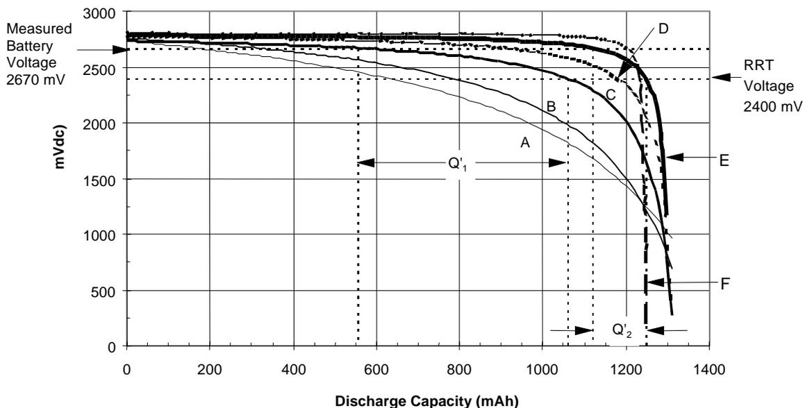
NOTE—Curve A = 800  $\mu\text{A}$ , B = 400  $\mu\text{A}$ , C = 100  $\mu\text{A}$ , D = 50  $\mu\text{A}$ , E = 20  $\mu\text{A}$ , and F = 5  $\mu\text{A}$ .
