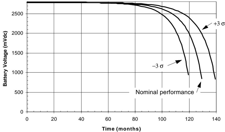
**Figure B.1—Example of projected longevity variability of a lithium/iodine battery**
