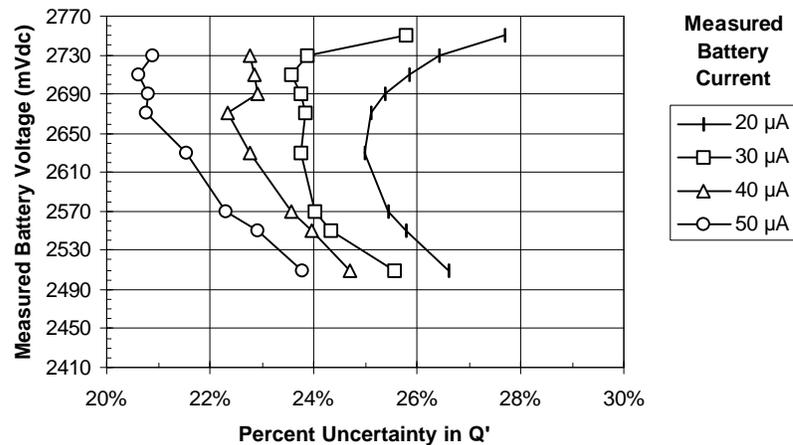
**Figure C.7—Percent uncertainty in Q' due to measurement error sources**
