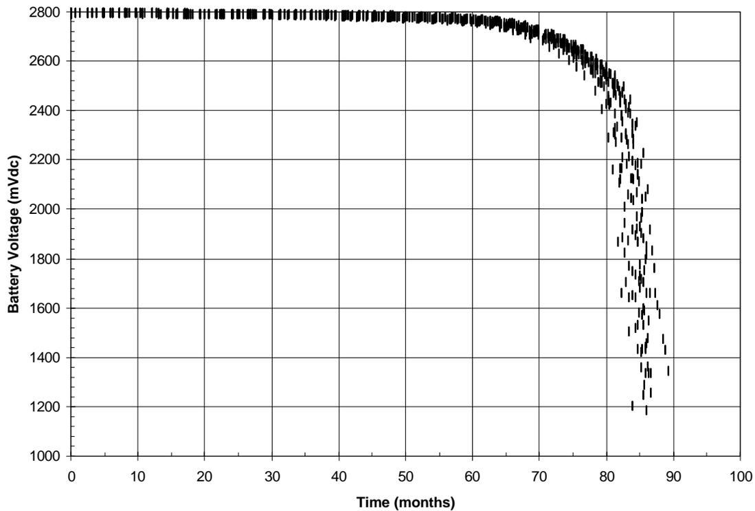
**Figure B.2—Discharge curves of a group of batteries discharged under a 12.5 K $\Omega$  load.**
