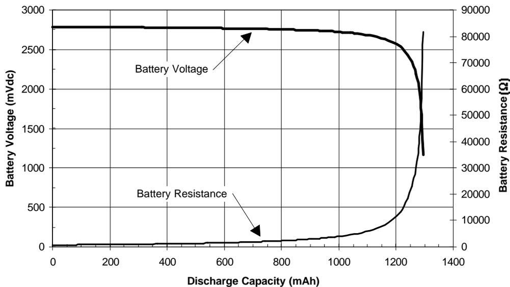
**Figure A.7—Relationship between voltage, internal resistance, and capacity for a specific lithium/iodine battery at a constant discharge current**
