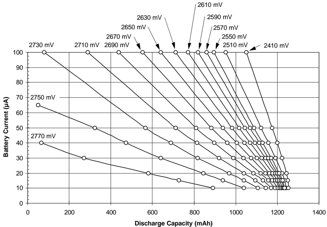
**Figure C.5—Battery current-capacity for a specific lithium/iodine battery**
