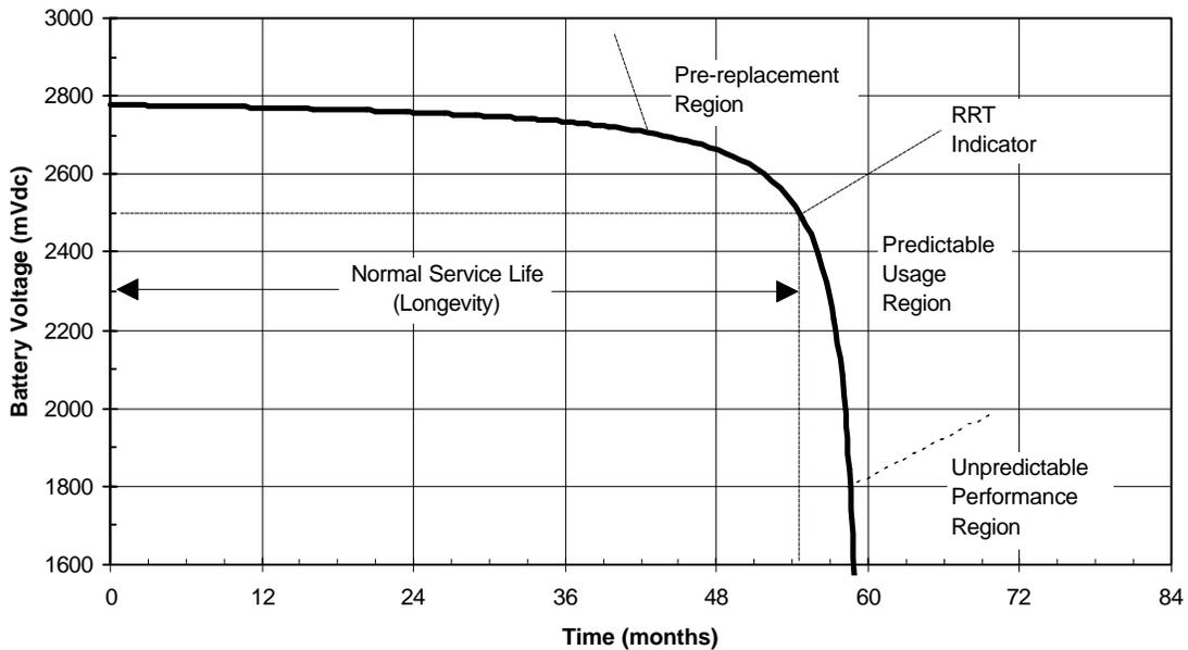
**Figure 1—Generic battery depletion curve**
