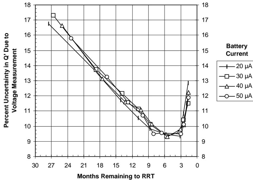
**Figure C.4—Percent uncertainty in Q' due to voltage measurement**
