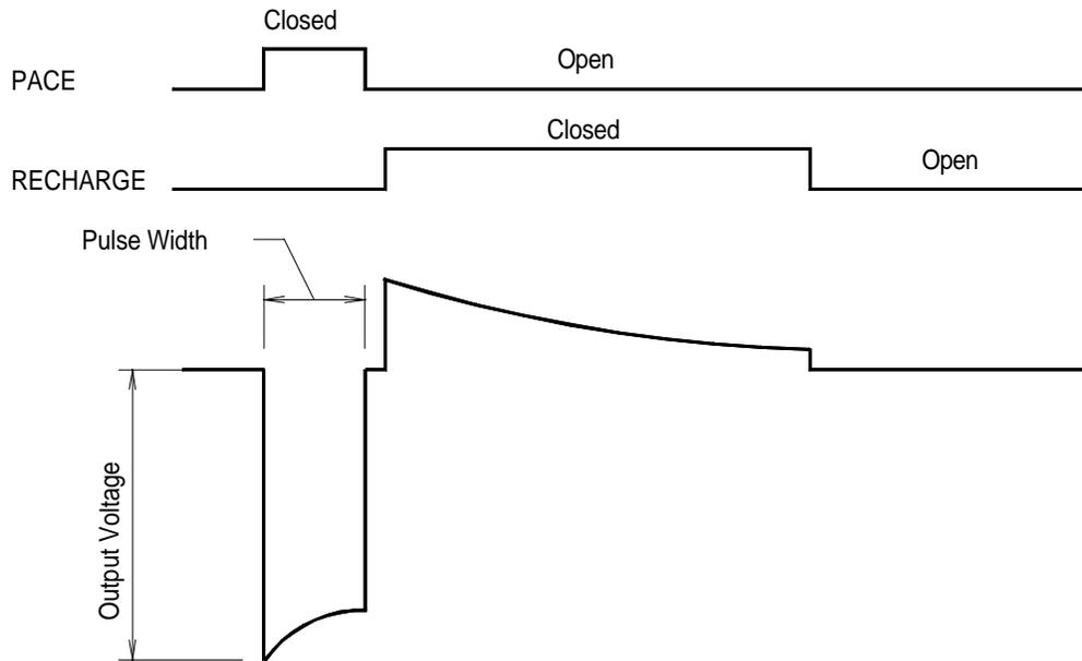
**Figure A.2—Typical constant-voltage pulse waveform**
