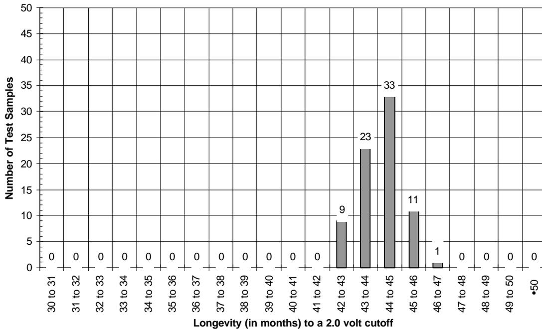
**Figure B.3—Life test results for a group of 77 batteries discharged under 100 KΩ constant resistive load**
