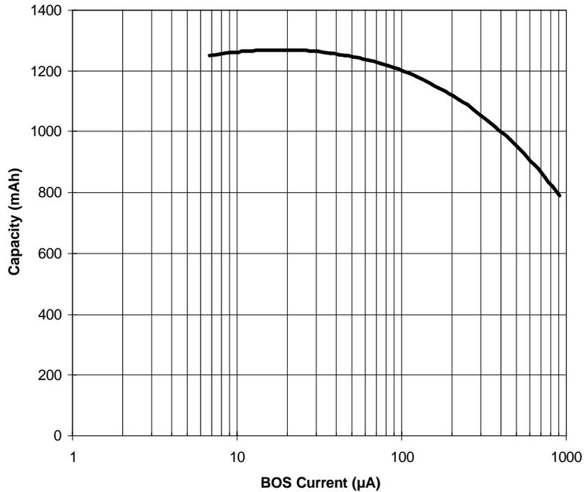
NOTE—BOS current refers to the current drain at the beginning of battery discharge. A cutoff voltage of 1.8 volts is assumed.
