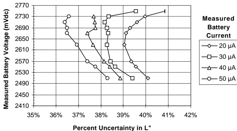
**Figure C.8—Percent uncertainty in  $L''$  due to measurement error sources**
