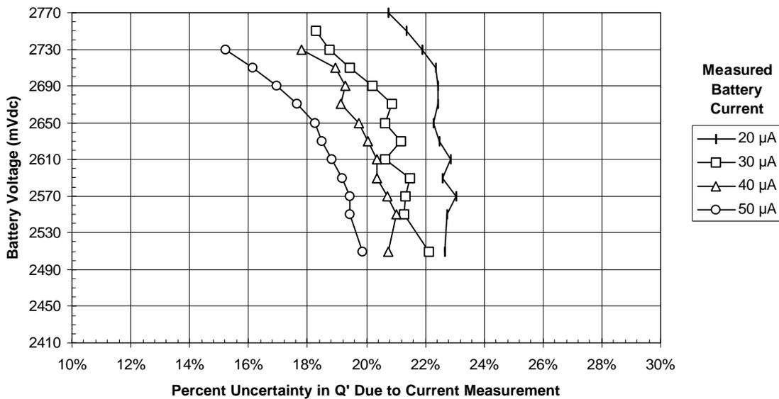
**Figure C.6—Percent uncertainty in  $Q'$  due to current measurement**
