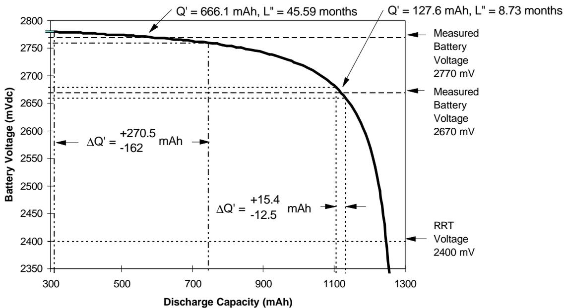
**Figure C.2—Load voltage–capacity for a specific lithium/iodine battery discharged at 20  $\mu$ A**
