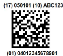
Figure 5.1-6. GS1 DataMatrix barcode
