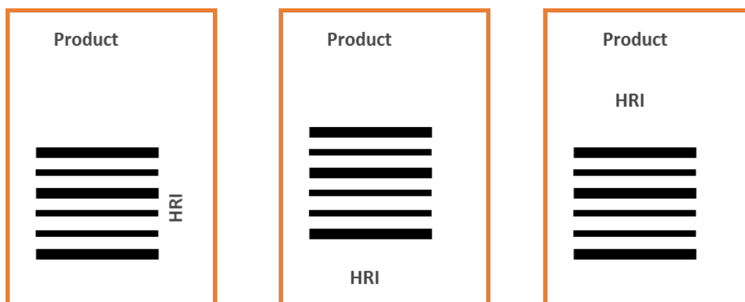
Figure 4.15-3. Locations of HRI for barcode in ladder orientation
