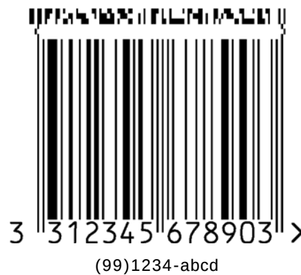
Figure 5.9.8-1. EAN-13 symbol with a four-column CC-A component
