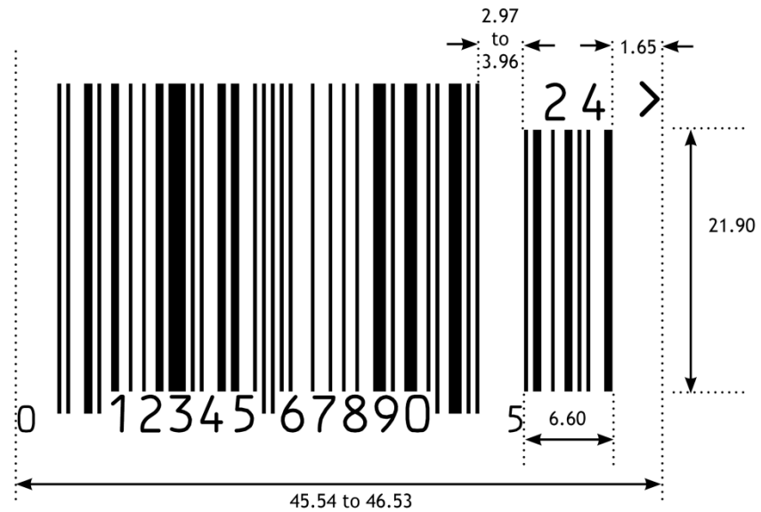
Figure 5.2.6.6-5. UPC-A barcode with two-digit add-on symbol
