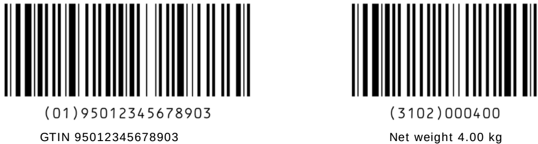
Figure 7.8.5.1-2. Data encoded in one concatenated GS1-128 symbol
