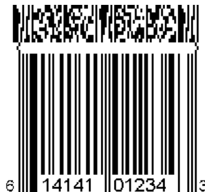
Figure 5.9.8-2. UPC-A symbol with a four-column CC-B component
