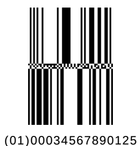
Figure 5.5.2.1.4-1. GS1 DataBar Stacked Omnidirectional barcode
