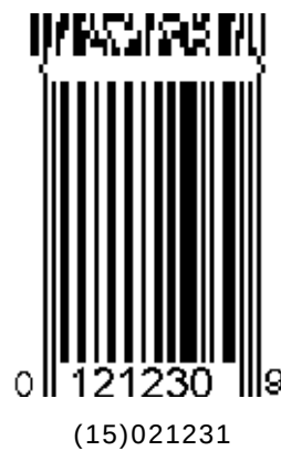
Figure 5.9.8-4. UPC-E symbol with a two-column CC-A
