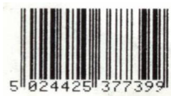
Figure 5.10.5.12-1. Symbol with edge determination problem
