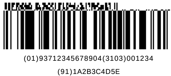
Figure 5.9.8-8. GS1 DataBar Expanded symbol with a four-column CC-A
