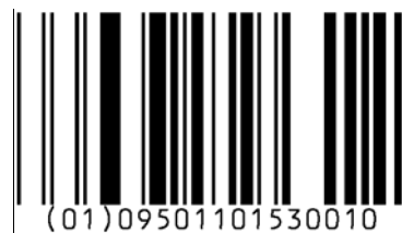
Figure 5.5.2.1.1-1. GS1 DataBar Omnidirectional barcode
