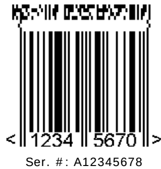
Figure 5.9.8-3. EAN-8 symbol with a three-column CC-A
