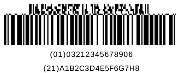
Figure 5.9.8-9. GS1-128 symbol with a four-column CC-A
