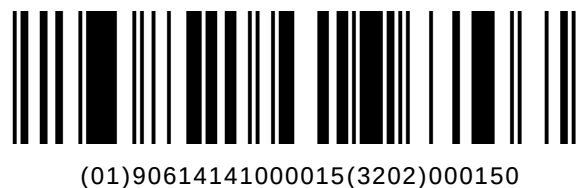
Figure 5.5.2.3.1-1. GS1 DataBar Expanded barcode
