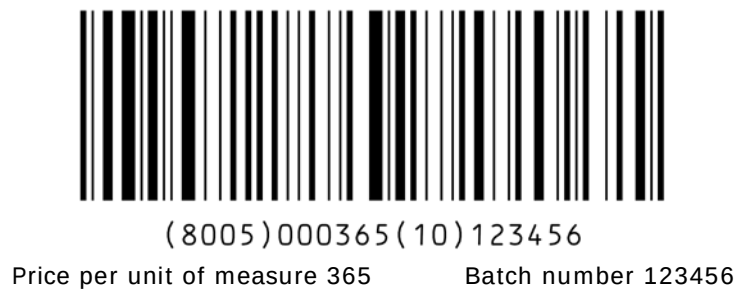
Figure 7.8.5.2-2. Data encoded in one concatenated GS1-128 symbol
