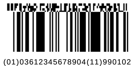
Figure 5.9.8-5. GS1 DataBar Omnidirectional symbol with a four-column CC-A
