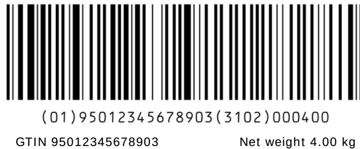
Figure 7.8.5.1-2. Data encoded in one concatenated GS1-128 symbol
