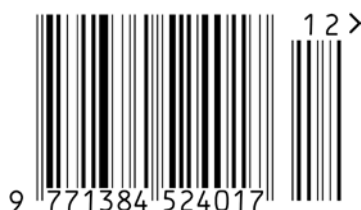
Figure 5.2.2.5.1-2. EAN-13 barcode with two-digit add-on symbol
