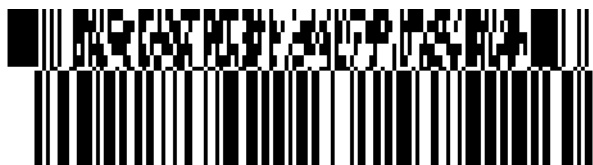
Figure 5.9.2-2. GS1-128 Composite symbol with CC-C
