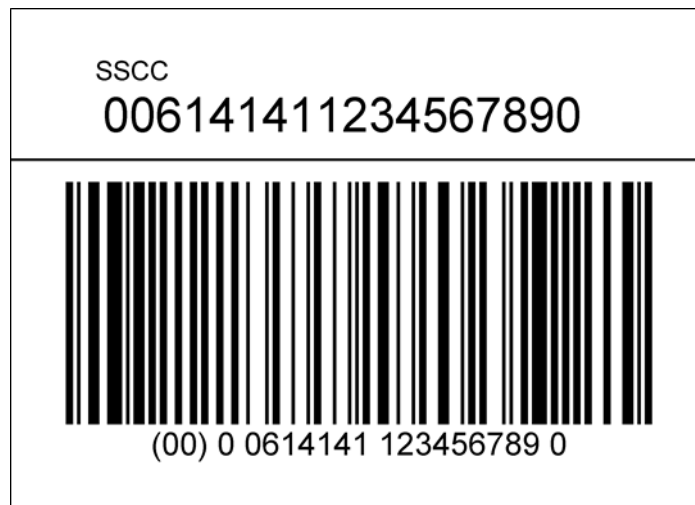
Figure 6.6.5-1. The basic label: an SSCC
