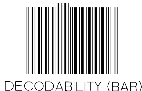
Figure 5.10.5.12-3. Calibration symbol with engineered low decodability grade
