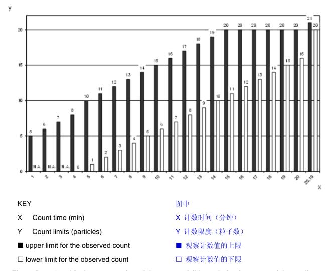
Figure D.2---Graphical representation of the pass or fail boundaries for sequential sampling
