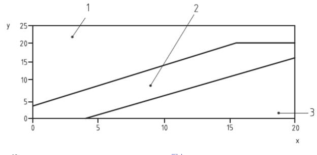
Figure D.1 — Boundaries for pass or fail by the sequential sampling procedure <br/>图D.1----顺序采样法合格与不合格的边界线
