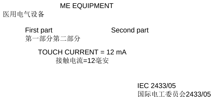
Figure A.11 – Interruption of a power-carrying conductor between ME EQUIPMENT parts in separate ENCLOSURES 图A.11-单独外壳中医用电气设备部件之间的载电导体中断
