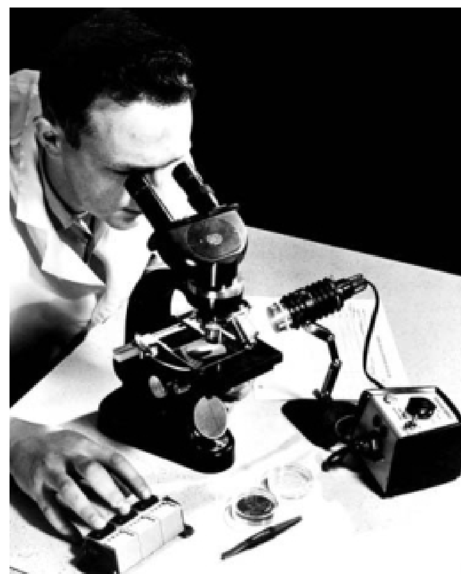
FIG. 6 Typical Counting and Sizing Microscope and Illuminator (see Test Method F25/F25M)
