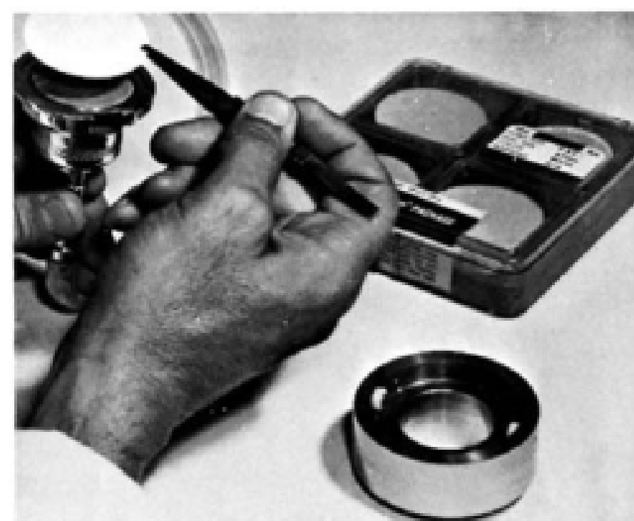
FIG. 5 Placing the Filter on a Typical Screen Support
