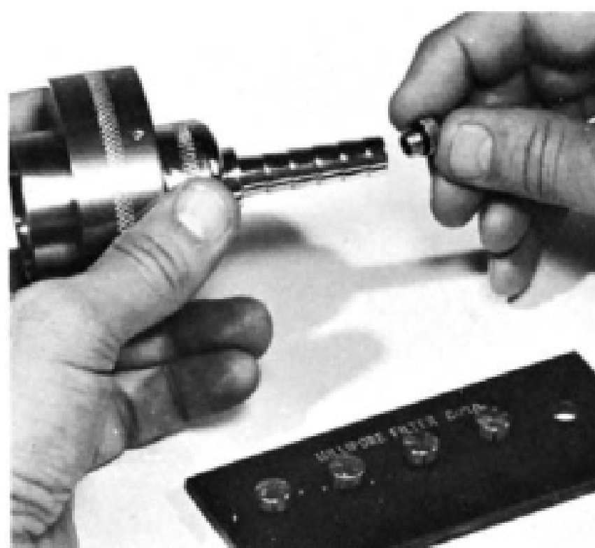
FIG. 4 Inserting a Typical Orifice
