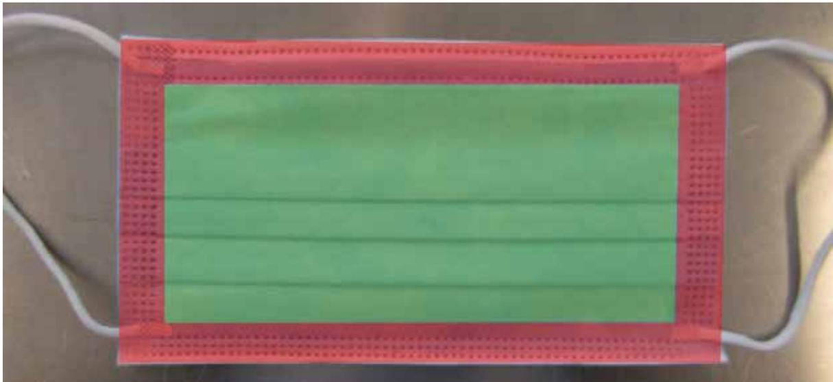
**Figure 2 - Main body (green) of the surgical/medical facemask must be tested for fluid resistance; the perimeter region (red) can be excluded from the testing.**
